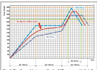
Fig. 5 IR reflow soldering profile for SMT process with SnAgCu series solder paste.
