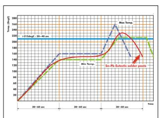
Fig. 6 IR reflow soldering profile for SMT process with eutectic SnPb solder paste.
